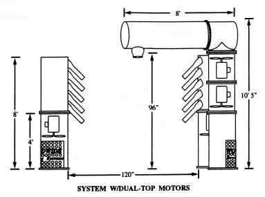
Motors: TEFC, 1.3 Service Factor, 3550 RPM. Factory extended leads.
