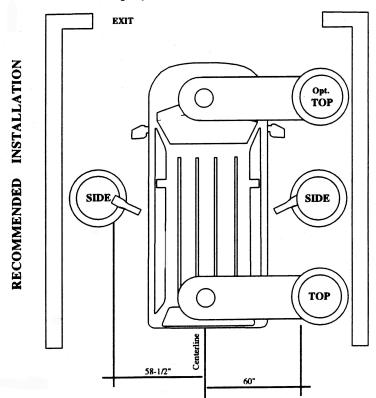
\*Recommend two feet (2') between side column base and top duct motor base.
